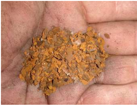
\text{Fe}_2\text{O}_3 Roest – Rouille (Hematite)
