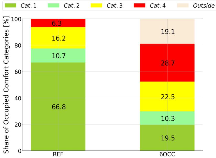
Figure 19: Comparison of thermal comfort categories time shares of operative temperatures for REF and 6OCC.
