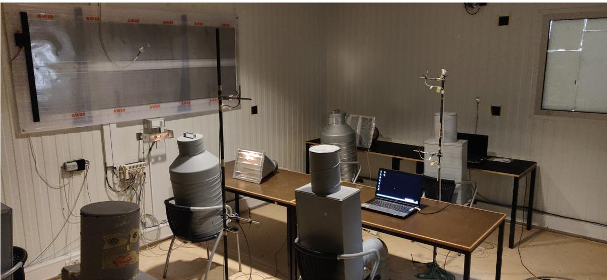
Figure 7: Picture of heat gain devices in chamber 6.
