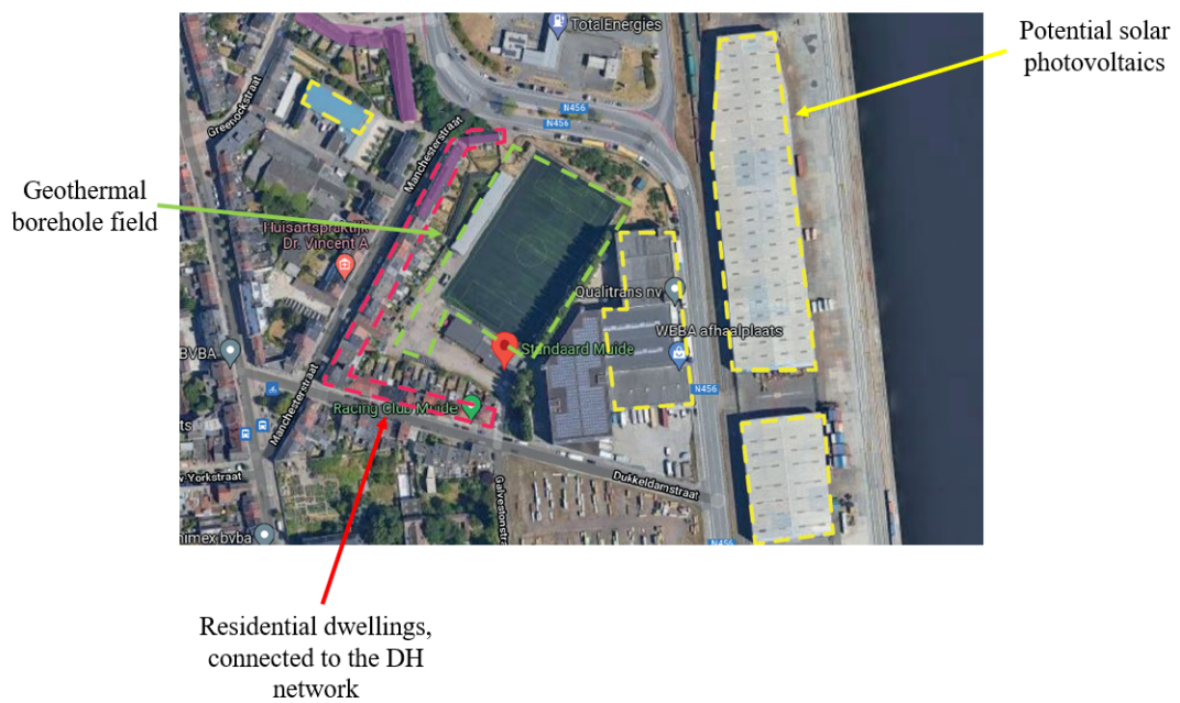
Figure 1.1: Overview of the district heating network in Ghent: the residential dwellings connected to the network (red), the area for geothermal heat extraction (green), the potential for the installation of solar photovoltaics (yellow).
