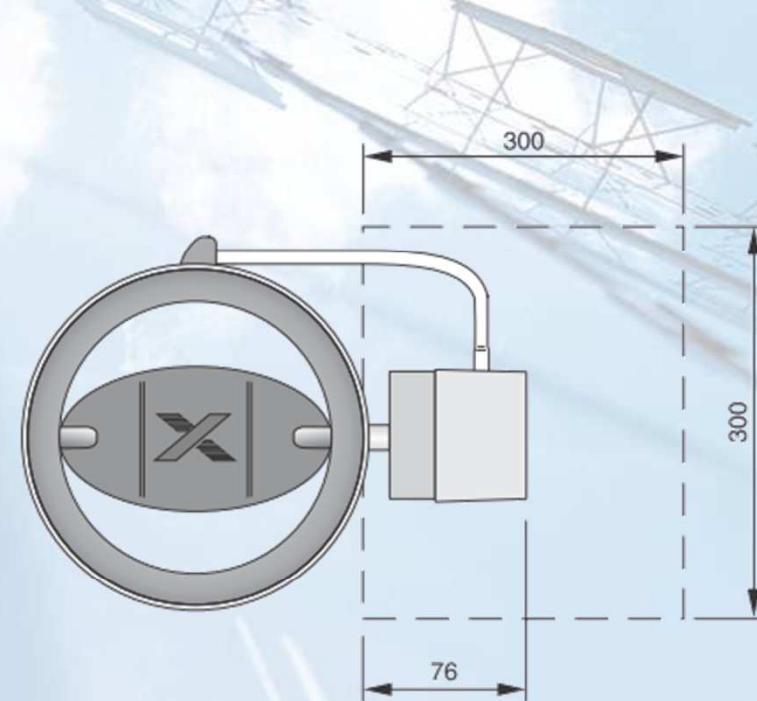
— — — Keep clear to provide access to control components
